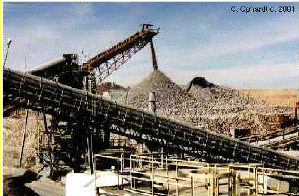
Various preliminary and intermediate stages of ore crushing leading to rotating mills in the plant
